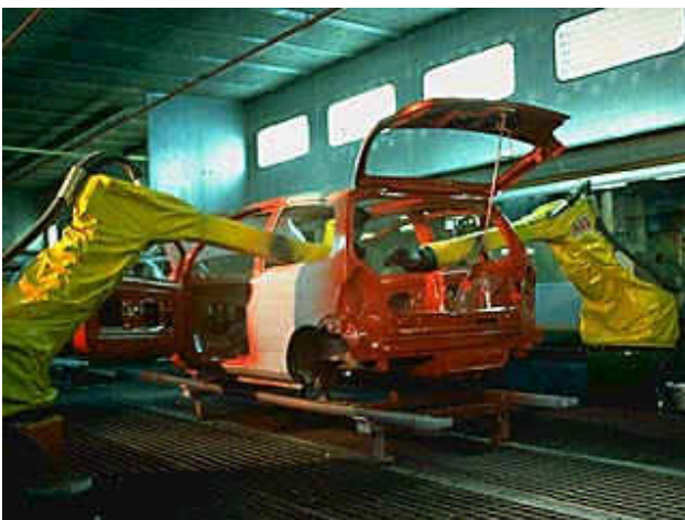
Body panels being painted by industrial robots.
